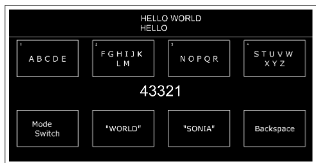
Figure 1: The user interface for our system. The target and currently typed text are displayed at the top. The selected character groups in the current word are shown in the middle of the screen, surrounded by the eight target boxes.
