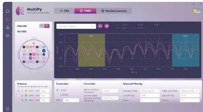
Figure 1 GUI of MultiPy in the fNIRS module, showing channel selection, real-time data visualization and available preprocessing options.
